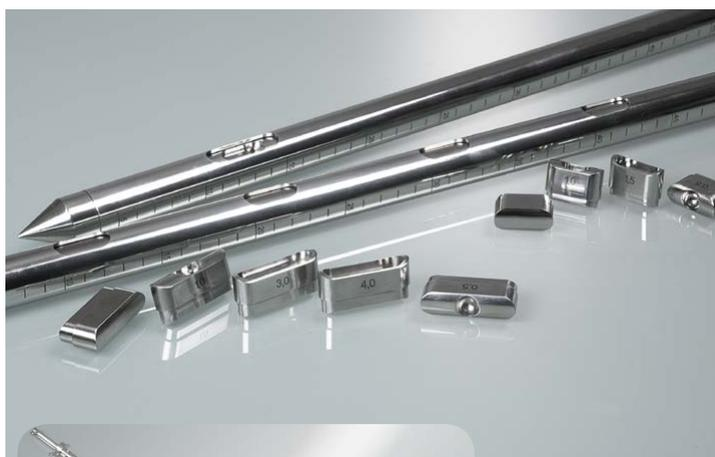
Novartos, the Pharma zone sampler for sampling according to FDA guidelines for Unit-Dose-Sampling. It is now possible to withdraw a triple-sample without inserting the lance repeatedly into the bulk material. Mixing is mainly prevented in this way. One significant advantage of Novartos is the easy cleaning. Complete filling and emptying of sample chambers has been improved substantially using computer-optimised geometry. There are no crevices or dead spaces where sampling residues can collect.
