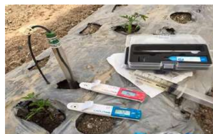
Figure 5: pH and conductivity testing on soil solution.
