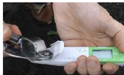
Figure 4: Placing sap directly onto LAQUAtwin nitrate sensor.
