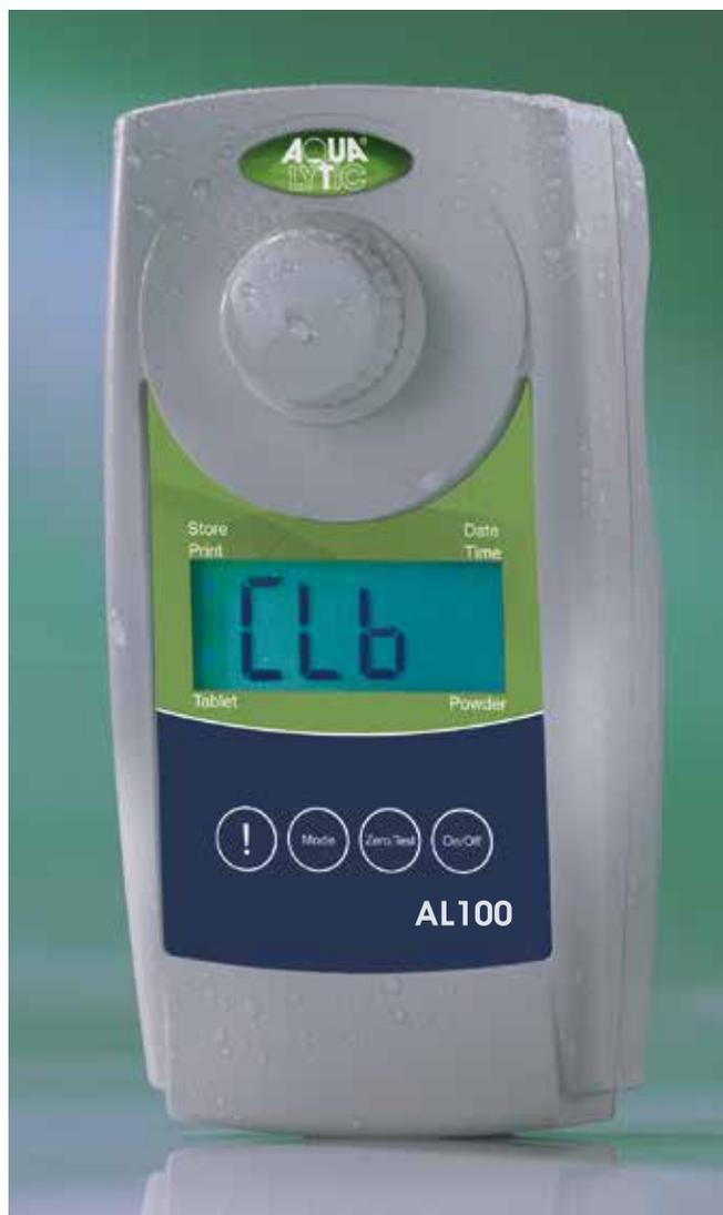
The AL100 uses high quality interference filters with long-life LEDs as a light source without any moving parts in a transparent sample chamber.
