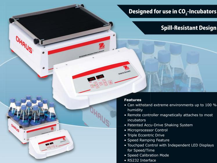
Ideal for applications that require CO<sub>2</sub> and humidity for optimal cell growth, the Extreme Environment Shaker is designed for use in extreme environments such as CO<sub>2</sub> incubators. A remote controller allows for external control of settings without disturbing the incubator atmosphere, and the shaker base is placed inside of the incubator.
